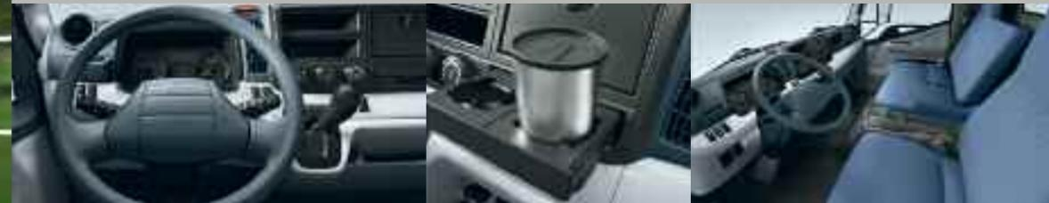
Automated manual transmission with dash-mounted shifter.
