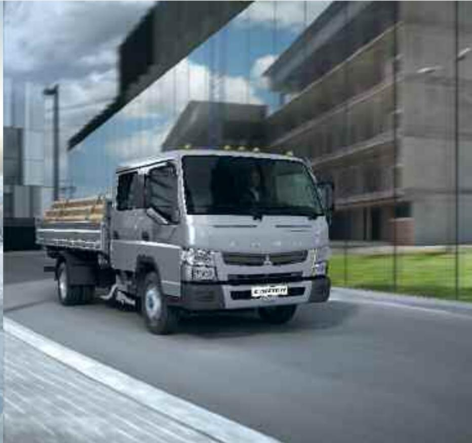
The Canter **FE130, FE160 and FE180** (13,200 lb., 15,995 lb. and 17,995 lb. GVWR respectively) set new industry standards for operational efficiency and driving ease. The Canter is the first medium-duty vehicle to feature a brake override system, dash-mounted shifter and a DUONIC® automated manual transmission that combines the efficiency of a manual transmission with the convenience of an automatic for unrivalled control and economy.
